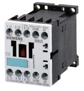
CONTACTOR, AC-3 3 KW/400 V, 1 NC, AC 230 V, 50/60 HZ, 3-POLE, SIZE S00, SCREW CONNECTION
