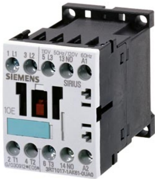
CONTACTOR, AC-3 4 KW/400 V, 1 NC, AC 110 V, 50/60 HZ, 3-POLE, SIZE S00, SCREW CONNECTION
