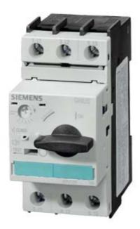
CIRCUIT-BREAKER SIZE S0, FOR MOTOR PROTECTION, CLASS 10, A-REL. 9...12.5A, N-REL. 163A SCREW TERMINAL, STANDARD SWITCHING CAPACITY
