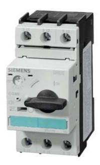
CIRCUIT-BREAKER SIZE S0, FOR MOTOR PROTECTION, CLASS 10, A-REL. 11...16A, N-REL. 208A, SCREW TERMINAL, STANDARD SWITCHING CAPACITY
