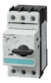
CIRCUIT-BREAKER, 14...20 A, N-RELEASE 260 A, SIZE S0, MOTOR PROTECTION, CLASS 10, SCREW CONNECTION STANDARD BREAKING CAPACITY,
