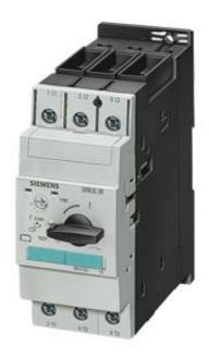
CIRCUIT-BREAKER 18...25 A, N-RELEASE 325 A, SIZE S2, MOTOR PROTECTION CLASS 10 SCREW CONNECTION STANDARD BREAKING CAPACITY
