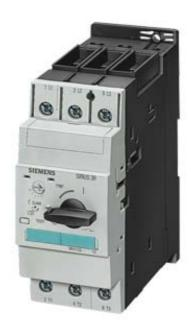
CIRCUIT-BREAKER SIZE S2. FOR MOTOR PROTECTION, CLASS 10, A-REL. 22...32A, N-REL. 416A, SCREW TERMINAL, STANDARD SWITCHING CAPACITY
