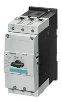
CIRCUIT-BREAKER SIZE S3, FOR MOTOR PROTECTION, CLASS 10, A-REL. 45...63A, N-REL. 819A, SCREW TERMINAL, STANDARD SWITCHING CAPACITY
