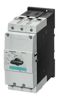
CIRCUIT-BREAKER SIZE S3, FOR MOTOR PROTECTION, CLASS 10, A-REL. 57...75A, N-REL. 975A, SCREW TERMINAL, STANDARD SWITCHING CAPACITY
